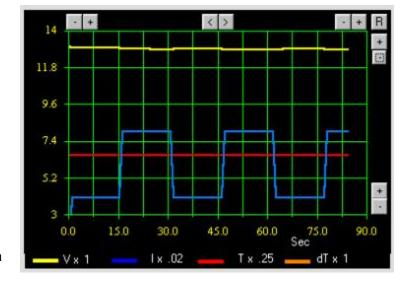
factor in the *Options-Graph* tab. All the data that is plotted on the graph is multiplied by this Y axis scale factor when plotted. Adjust the scale factors as required to make the plot lines easier to view. You will see the corresponding scale factor listed in the graph legend for your convenience.
