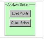
When using the *Load Profile* or *Quick Select* method the user does not need to concern themselves with selecting the correct charging algorithm for constant current or constant voltage. The BA400 will automatically select this for you once you select the battery type.
