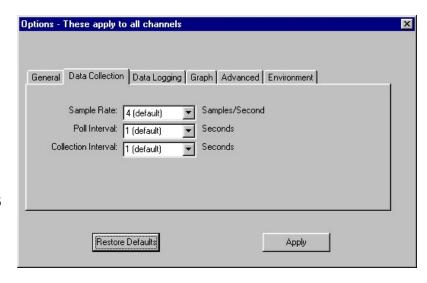
When using multiple analyzers you may wish to increase the poll interval (decreased the frequency) in order to relive the PC and speed up the software response time.
