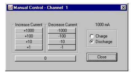
There may be instances when you want to be able to collect data using a manual control. This allows you to adjust the current in real time. Using this feature you can create charge or discharge currents of any value.
