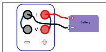
Analyzer with a 4 wire option being used in a 2 Wire mode. Note the jumpers connecting each pair of terminals. The I and V inputs are externally connected in this case. Ensure that these jumpers are securely fastened. This configuration is suitable for many applications.
