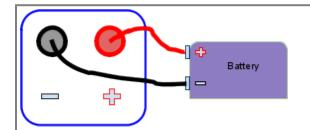
Standard 2 Wire configuration. There are only 2 leads required. The I and V inputs are internally connected. At high current, the voltage at the battery terminals can deviate slightly from the voltage appearing at the analyzer input. In most cases this is insignificant and can be ignored.
