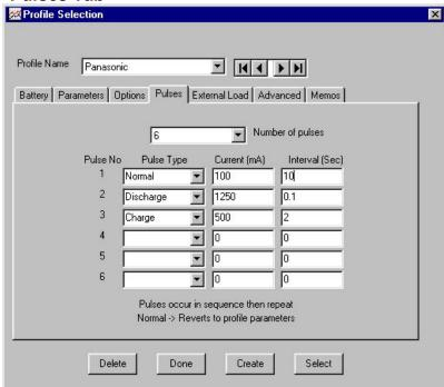
Using the pulse feature of the BA400 you can overlay pulses of various currents and duration on top of the normal discharge or charge current. This feature allows you to simulate real load conditions or develop special charging and discharge procedures.
