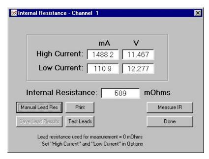
Batteries have an Internal Resistance (IR) that causes a voltage drop when current is drained from battery. The IR also causes the terminal voltage to rise when current flows into the battery during charge.
