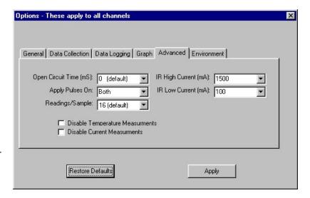
Off - Disables all pulses, Discharge - Pulse activated during discharge only, Charge - Pulses activated during charge only, Both - Pulses activated during all discharges and charges.
