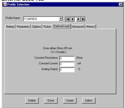
This tab is used to control the optional external load modules. These optional modules can be used to increase the discharge current during tests. These can be used to shorten the discharge time for large capacity batteries or to increase the pulse discharge current for load tests.
